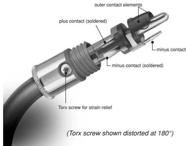
But your nextgen plug WBT-0110 makes it even more comfortable: By pressing the two snap hooks left and right you have the possibility to pull out the whole Central Contact Unit by the front. This way you may solder the plus and the minus outside the connector's body.
